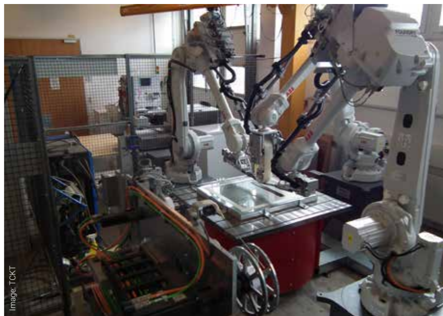
Automated tape laying
