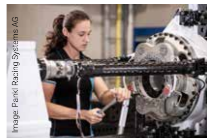
Validating lightweight components on the engine and drivetrain test beds.
