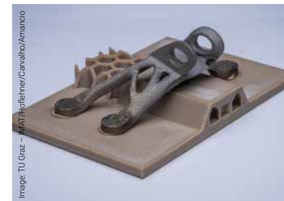
Ultrasonic Joining of FFF-PEEK with LPBF 316L stainless steel
