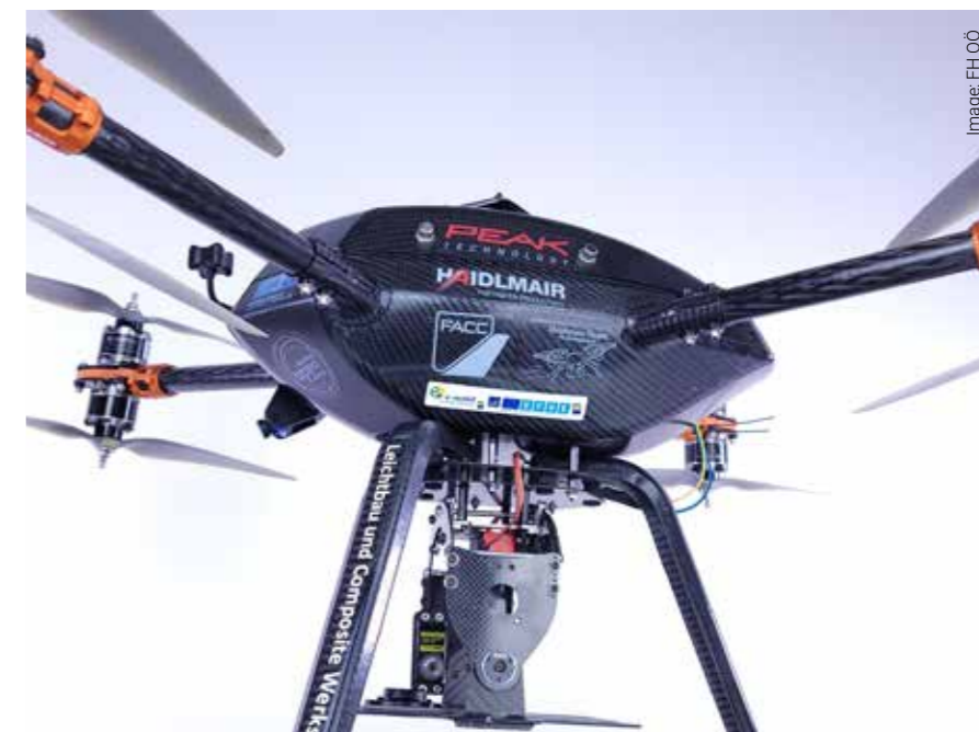
Weight-saving, high-strength composites are the ideal material for drones. Students at the University of Applied Sciences Upper Austria applied their know-how and expertise in lightweight design to develop a camera drone in a very integral design and enable a weight saving of more than 40 %.
